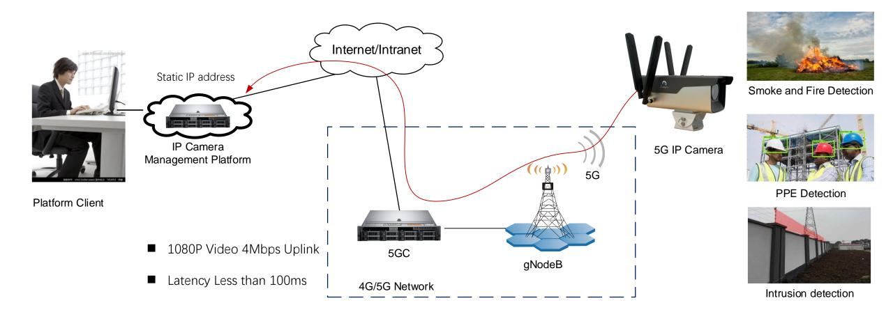
Xingtera provide 5G IP camera and camera backend management platform end to end solution
