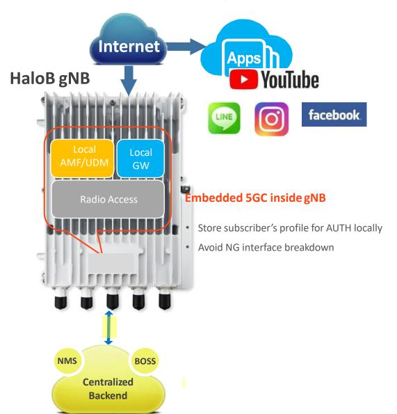
Put a lite 5G Core inside gNB to make the whole system more robust and easy deploy
